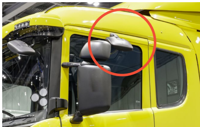
Class V mirror to be fitted to the nearside
