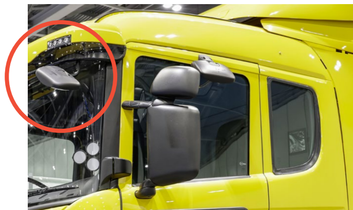
Class VI mirrors to be fitted to the front
